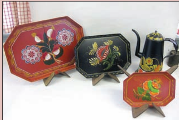
Prior to 1835, tin sheets did not exceed dimensions of 10 by 14 inches. The center tray is one full sheet. In front is a tray composed of half a sheet, and the tray in back, as well as the coffee pot, are made with two sheets fused together.
